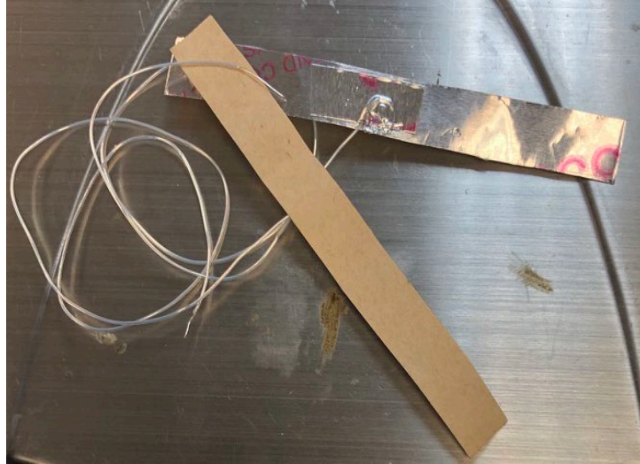
Figure 6. Image of the antenna used to measure impedance. Each antenna is approximately 80 mm x 10 mm x .20 mm. The back section peels off and the adhesive material attaches to the ThinSat frame.
