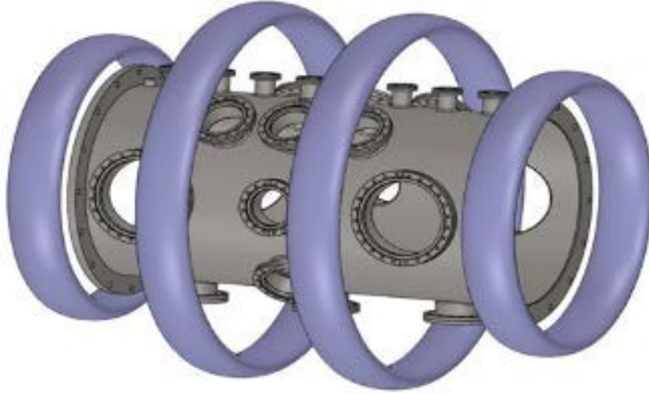
Figure 9. Cartoon of a plasma chamber with electromagnets surrounding the chamber. The spacing and size of the electromagnets was determined to provide a uniform magnetic field throughout the entire chamber.
